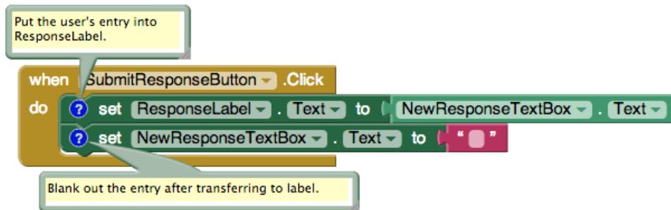
**Figure 4-4.** Setting the response to the user's entry
