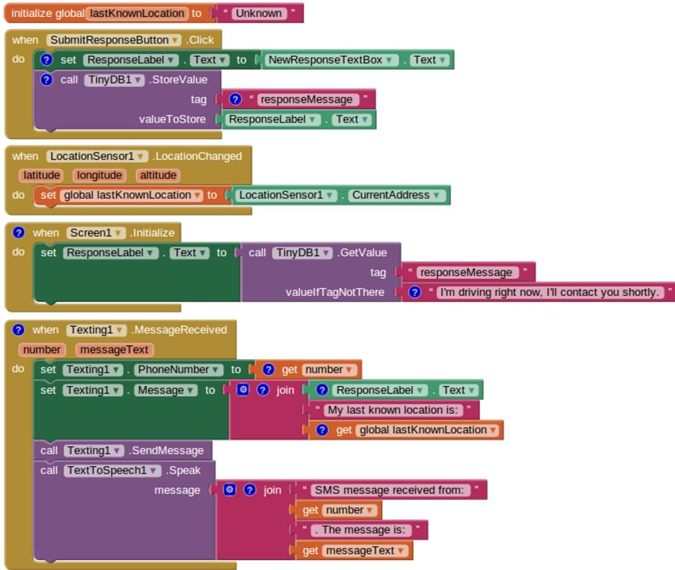
Figure 4-11. The complete No Texting While Driving app
