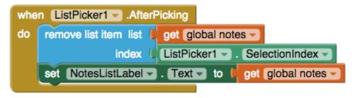
Figure 19-20. Removing an item by using ListPicker.SelectionIndex
