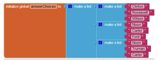
**Figure 19-22.** A list of lists is formed by inserting make a list blocks as items within an inner make a list block
