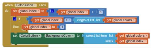
**Figure 19-10.** Using an if to check whether the index value is larger than the length of the list
