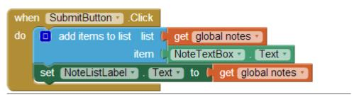
Figure 19-15. Displaying the list to the user by placing it in a label.
