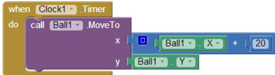
Figure 17-4. Moving the ball horizontally across the screen
