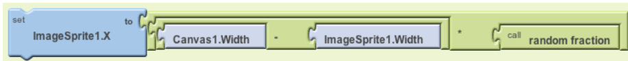
Figure 16-11. You can use math blocks to build complex expressions like this one
