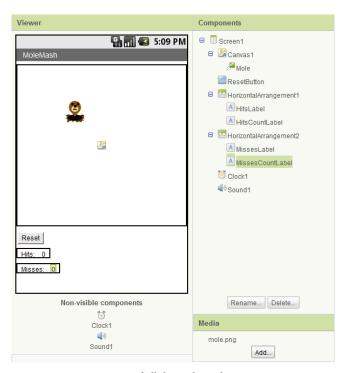
Figure 3-3. The Component Designer view of all the MoleMash components
