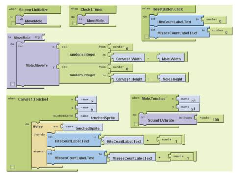
Figure 3-11. The complete MoleMash application
