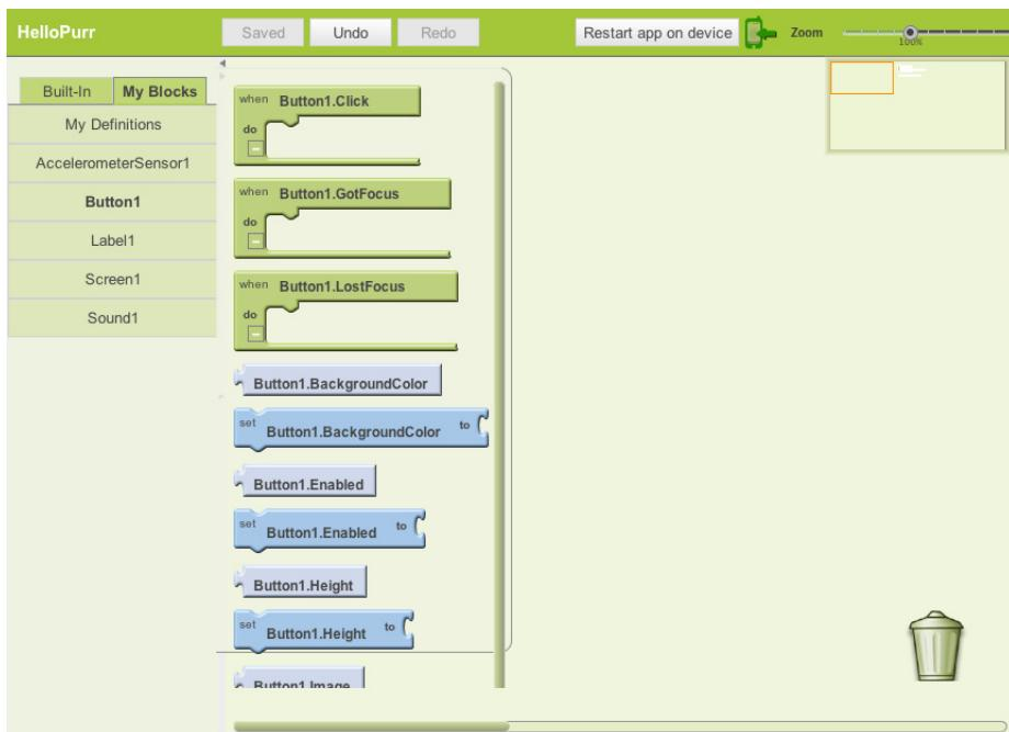
Figure 1-7. Clicking Button1 shows the component's blocks
